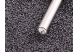
The tip of the sensor must be isolated from ground.
