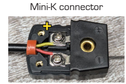
Properly installed Mini-K connector. Note: Yellow is +, Red is -
